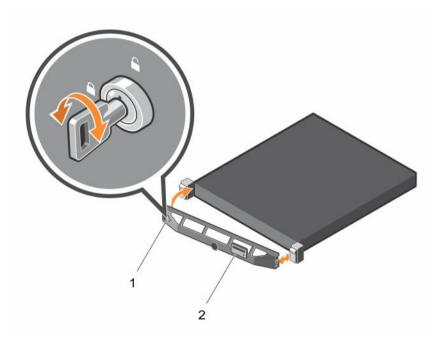
Figure 14. Removing and installing the Quick Sync bezel
